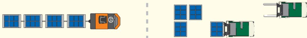
By towing loaded dollies linked in series, the CBT/CBTY can transport large loads at one time. A forklift must travel back and forth many times to transport the same load volume.
